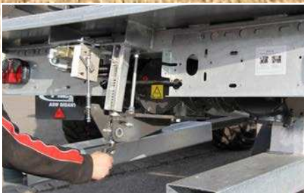
Push-off speed is adapted automatically by the automatic feed control
