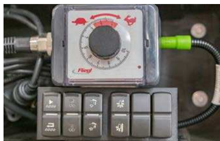
Control Block with Electric Potentiometer and Control Panel: Operation of hydraulic functions such as the conveyor floor drive, pressure flap, and rear wall. Infinitely variable speed regulation of the conveyor floor via a rotary knob in the tractor cabin. The control range and resolution can be redefined by the customer or a workshop.
