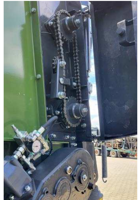
Milling Drum Connection via Chain (KDS 255)
