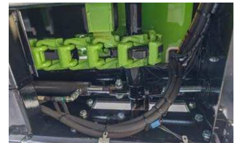
Hydraulic chain tensioning
