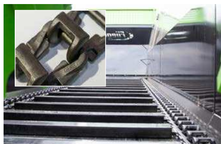
2 External Chain Strands: Made of V2 chain links with a breaking load of 50 tons.
