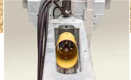
The spreading gear is driven mechanically by a PTO through-drive shaft
