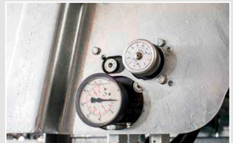
Mechanical potentiometer with adjustable feed rate at the spreading unit
