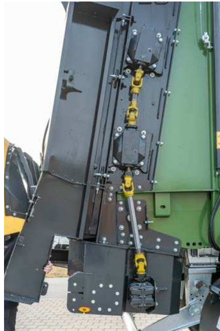
Milling Drum Drive via Cardan Shaft
