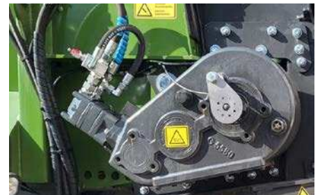
Conveyor Floor Drive: Spur gear and hydraulic motor located on the left side in the direction of travel.
