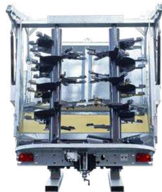
Milling drums with throwing vanes
