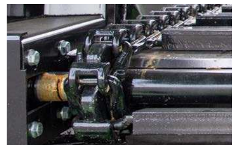
Star-Shaped Sprockets: Designed for low susceptibility to contamination.
