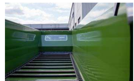
KDS 260: body made from fine-grain steel
