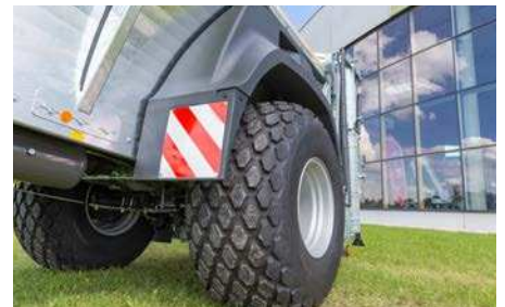
Optional: 40km/h version with mudguards with ADS 80 / ADS100 / ADS120
