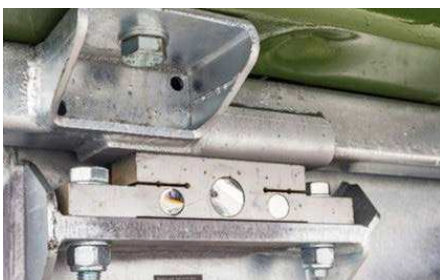
Weighing System: Precise determination of payload. In conjunction with the ISOBUS control system Spreader Control, the controller can regulate the conveyor floor speed based on weight changes.
