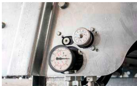
Mechanical feed control through mechanical potentiometer
