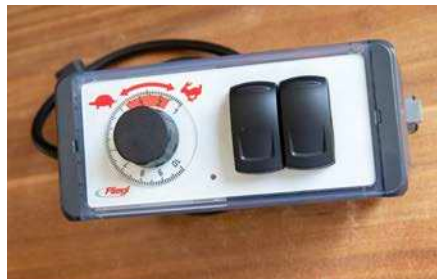
Electric Potentiometer with Dual Changeover Valve: Control of hydraulic functions for support leg/drawbar, pressure flap, and rear wall via a double-acting control unit. Infinitely variable regulation of the conveyor floor speed. The control range and resolution can be redefined by the customer or a workshop.
