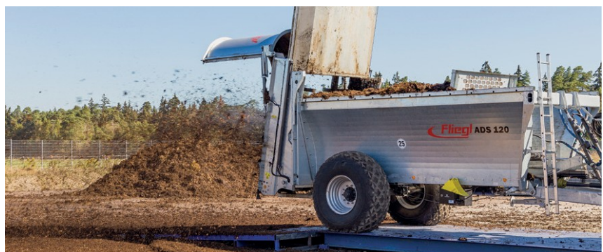
Figure 3: FLIEGL ADS 120 on the test stand for longitudinal distribution
