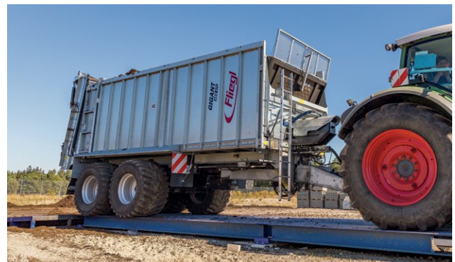
Figure 3: FLIEGL ASW 271 on the test stand for longitudinal distribution
