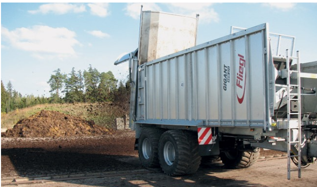
Figure 2: FLIEGL ASW 271 on the test stand for transverse distribution
