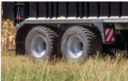
Bandenvarianten tot 800/45 R 22.5" of optioneel 710/50 R 30.5"
