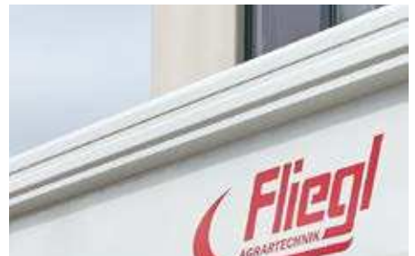
Reinforcement profiles bent and rounded from a single piece.
