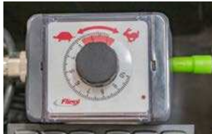
Electric Potentiometer: Infinitely variable adjustment of the conveyor floor speed via a control unit in the tractor cabin. The control range and resolution can be redefined by the customer or a workshop.
