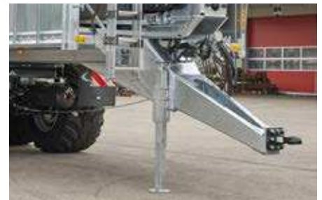
Drawbar unsprung, rotatable for Top and bottom attachment
