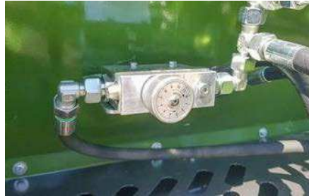
Mechanical potentiometer with feed rate adjustment at front of spreader body
