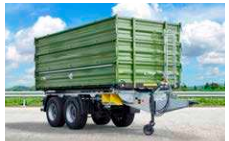
TDK 160 with 1800 mm body (3 x 600 mm tailgate)
