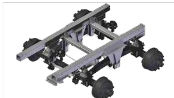
Titan tandem assembly for best ground adaptation, lubrication and maintenance free.
