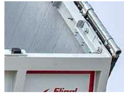
Double-joint hinge and dual hook locking system
