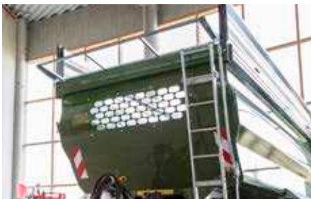
Mechanically folding protective grating
