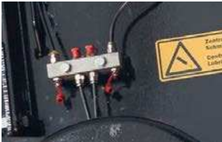
Central lubrication point
