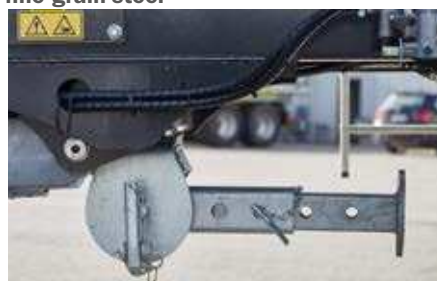
Supporting stand Adjustable, centrally rearward-folding for maximum stability
