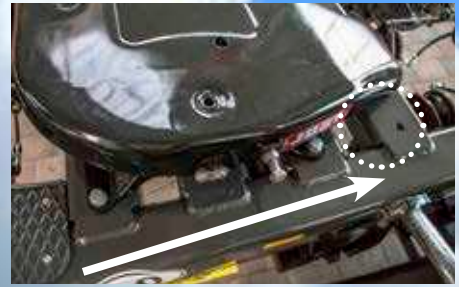
Mechanically adjustable fifth wheel plate for one-axle and tandem dolly
