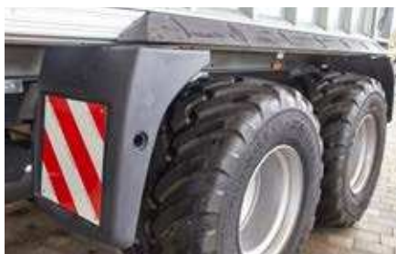
Mud guards and rear covers made of robust plastic parts guarantee clean surfaces and reduced risk of injury.
