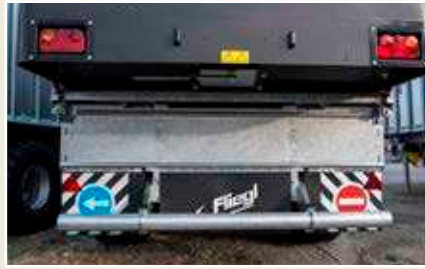
Germany 40 km/h version with fixed underride guard
