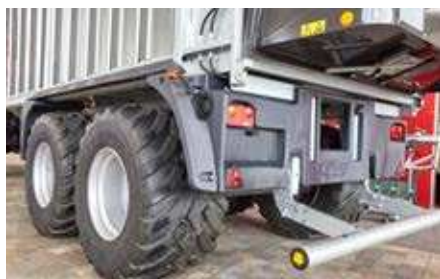
Mud guards and rear covers made of robust plastic parts guarantee clean surfaces and reduced risk of injury.
