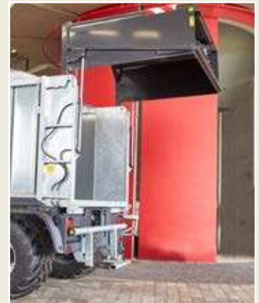
When the large-area back wall opens, the underride guard folds up automatically
