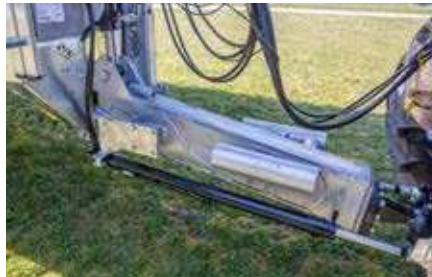
Hydraulic forced steering
