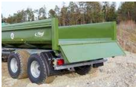
Gravel flap on models TMK 130 S and TMK 200 S.
