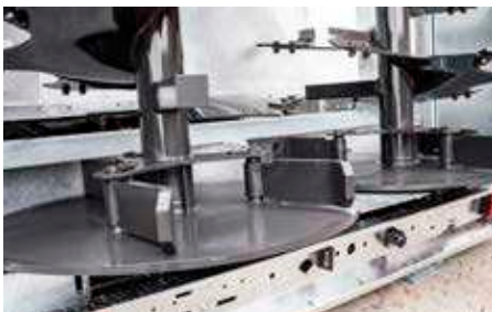
Spreading unit Profli V2 with slinger:
