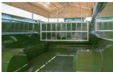
Chequer plate floor for animal safety
