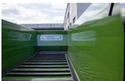
KDS 260: body made from fine-grain steel
