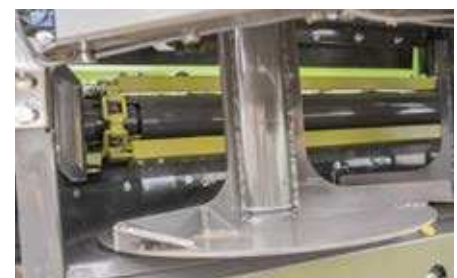
The conveyor floor consists of 2 flat link chains with continuous scraper bars.
