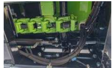
Hydraulic chain tensioning
