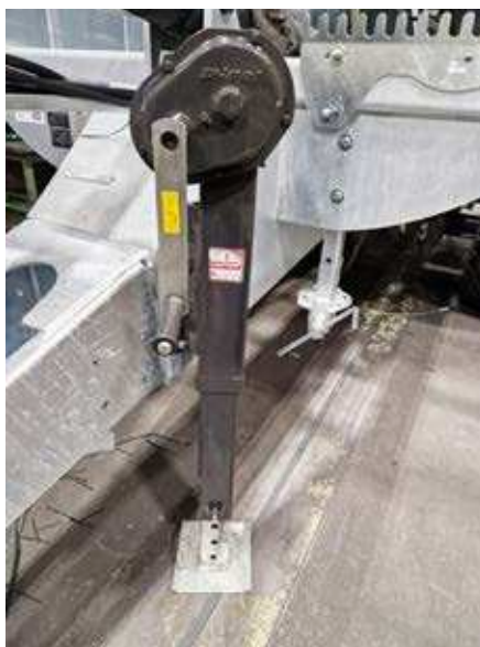
Drop support with 2 speeds
