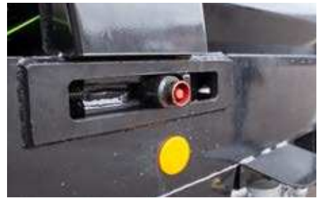
Easily accessible chain wheels which can be lubricated through the shaft on either side
