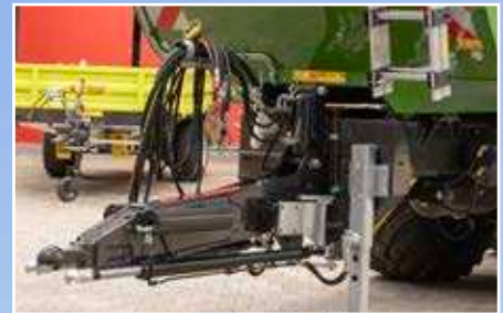
Hydraulically cushioned drawbar.
