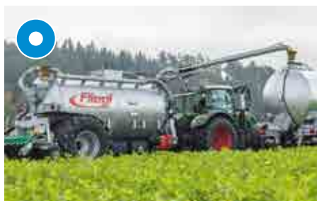
Hydraulisk svingbar sugearm 8"
