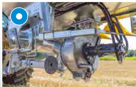
For vakumtankvogner: Turbofyllingsanord- ning midt under tanken – for lasting fra begge sider
