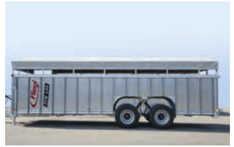
The TTW 140 Tandem Noah livestock transport trailer has a total length of 8.3 m
