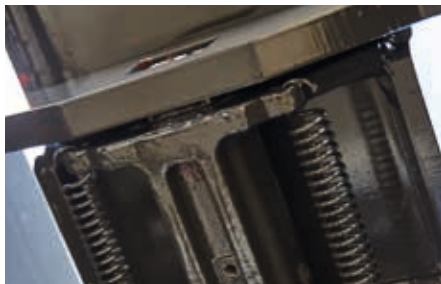
Automatic hook lock for tipping process
