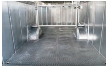
Chequer plate floor for animal safety
