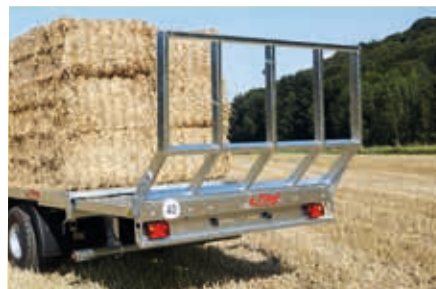
Bale grid for type DPW 180 B as standard Optional: rear extension (1200 mm)
