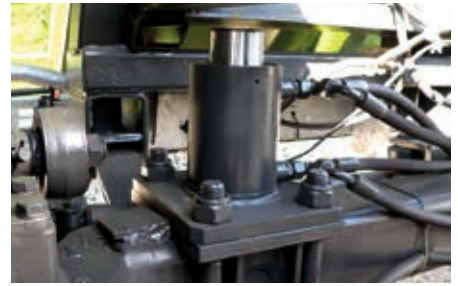
Optional: hydraulic support at the axle
