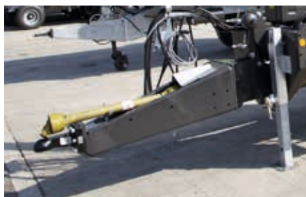
Swivelling drawbar for top and bottom hitch
