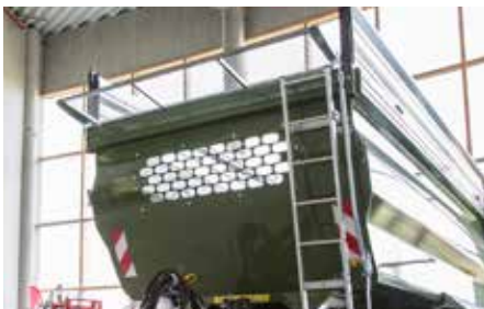
Mechanically folding protective grating
