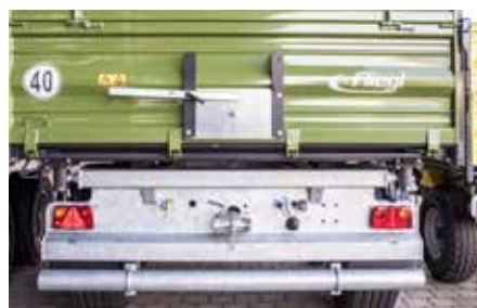
40 km/h version with underride guard and mudguards
