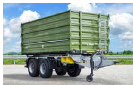
TDK 160 with 1800 mm body (3 x 600 mm tailgate)
