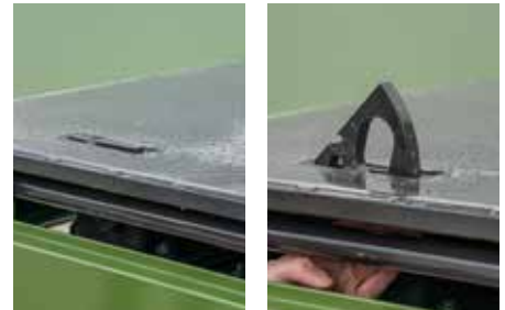
Retractable lashing eyes
