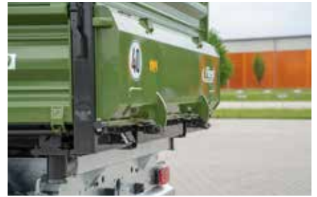
Robust flap with 2-cylinder design
