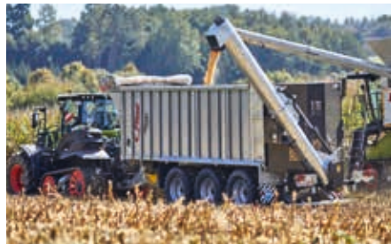
Overloading auger ÜLS 400 for grain Overloading rate about 7.5to/min
