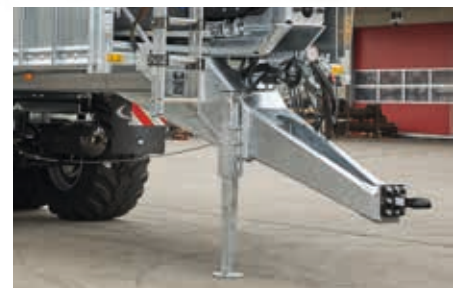
Drawbar unprung, rotatable for Top and bottom attachment
