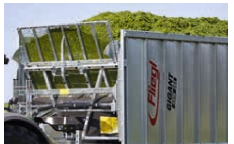
Sealing strips: Special polyurethane strips arranged at a 45° angle seal the loading area perfectly.
