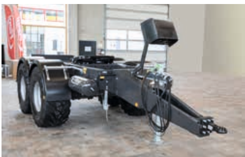
Tandem-Dolly with 17 t coupling load and 20 t total weight
