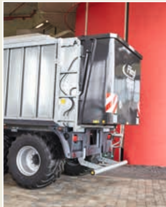
When the large-area back wall opens, the underride guard folds up automatically
