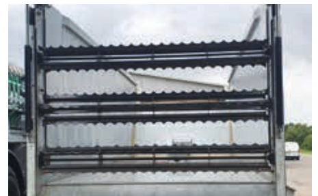
Dosing roller with 3 horizontal milling drums
