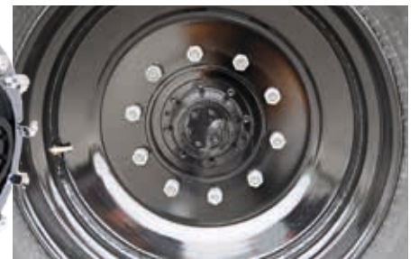
The radial piston motor provides additional drive power if required.
