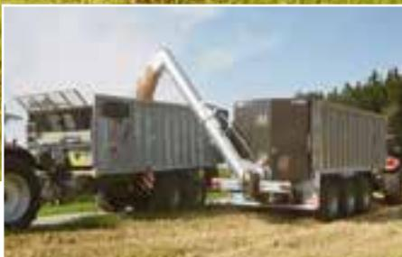
Overloading auger ÜLS 400 for grain
