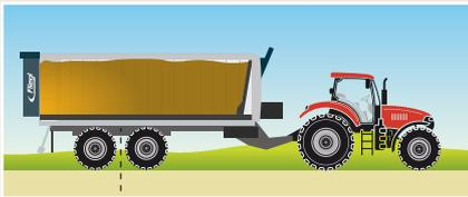
Optimal adaptation of drawbar load by mechanical axle shift (standard) or stepless hydraulic adjustment (as option)
