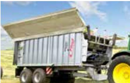
TOPLIFT: The two tarpaulin halves can be opened and closed in the shortest time
