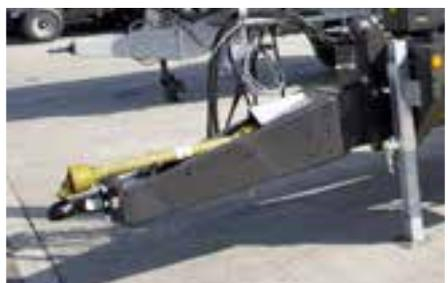
Swivelling drawbar for top and bottom hitch
