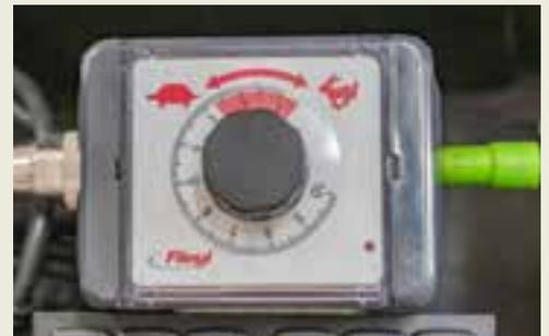
**Electrical potentiometer** with feed rate adjustment on control panel
