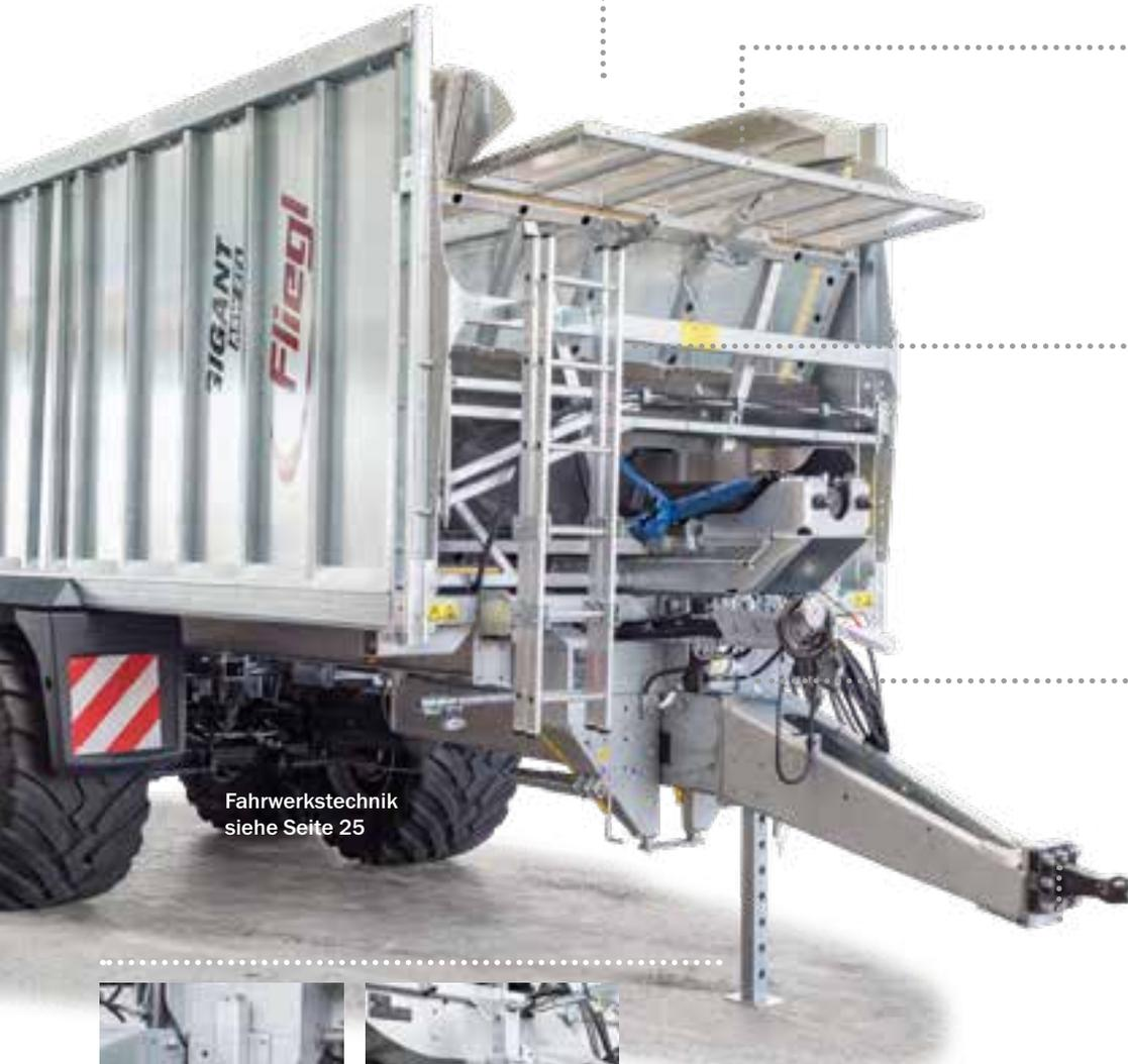
Grating extension: adjustable mechanically in the standard version, hydraulically adjustable as option.
