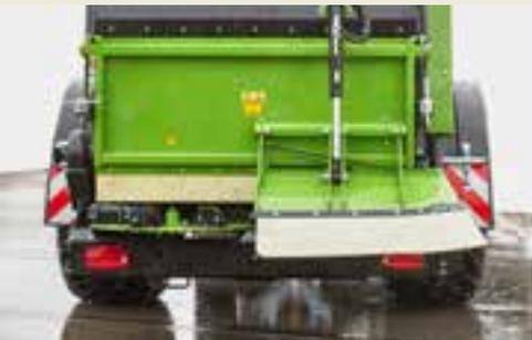
**Edge spreading device**
