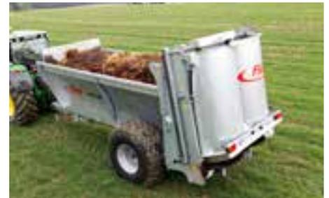
With the proven Fliegl push-off technology, the material is fed evenly to the spreading unit. When the spreading is over, the loading area is virtually clear and the underfloor remains clean, unlike with conventional scraper floors.
