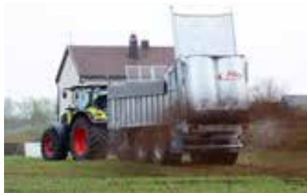
Spreader "Profi V2" with closed wide-spreading back wall
