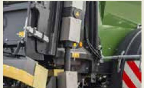
**Milling drum drive above drive shaft**
