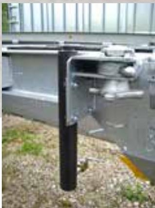
Cylinder for hydraulic lifting gear
