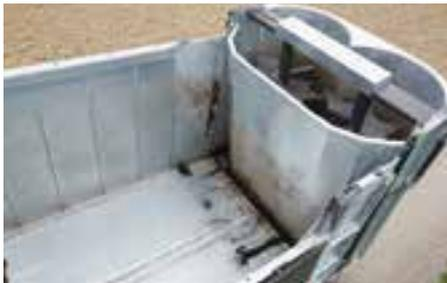
The sliding gate is fully galvanised as standard. The spreading unit bearings can be accessed through a central lubrication bar for easy maintenance.
