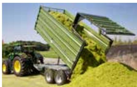
Silage tipper with hydraulic back wall
