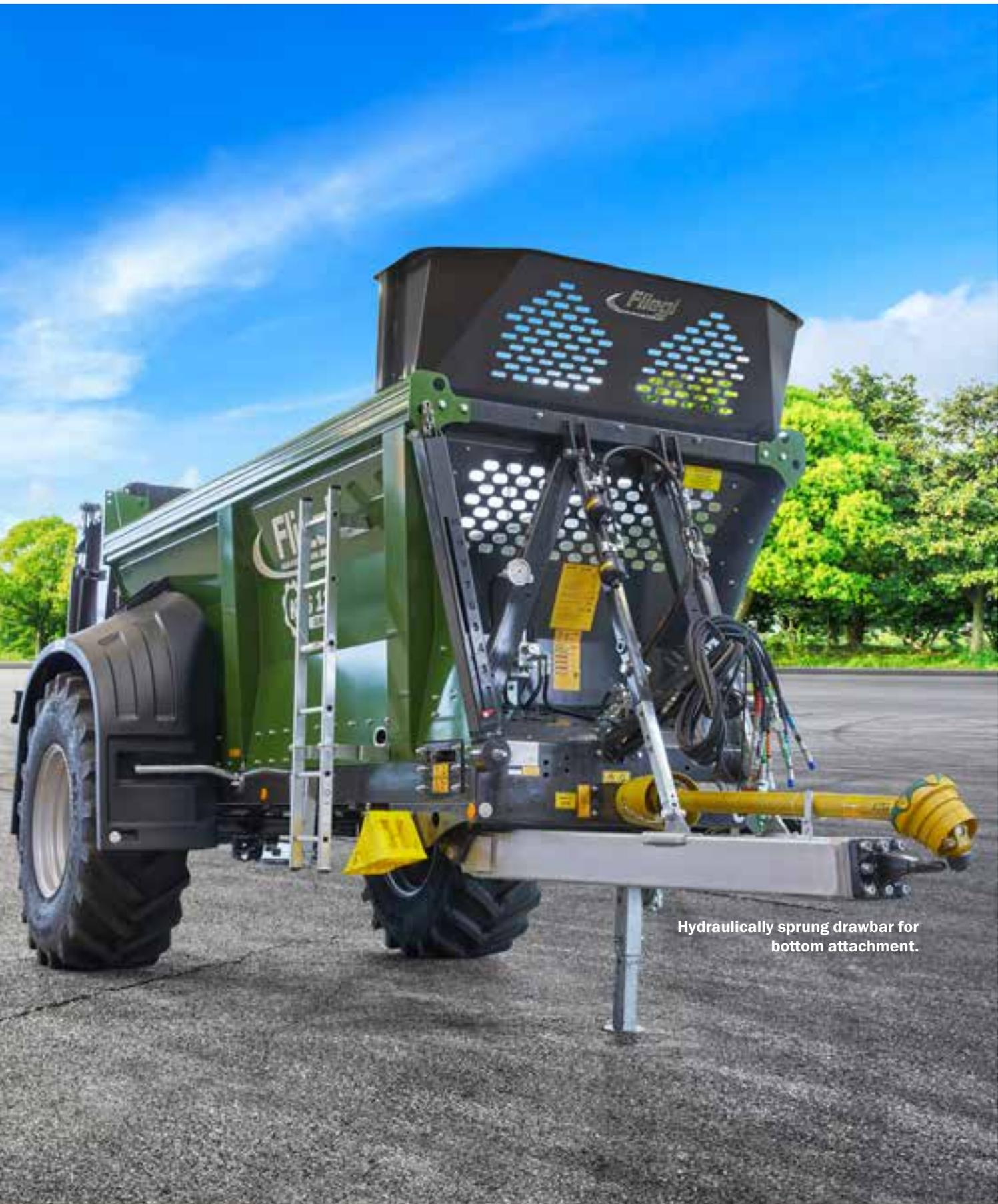
Hydraulically sprung drawbar for bottom attachment.
