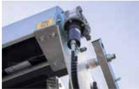
Protection guard to prevent dirt and damage
