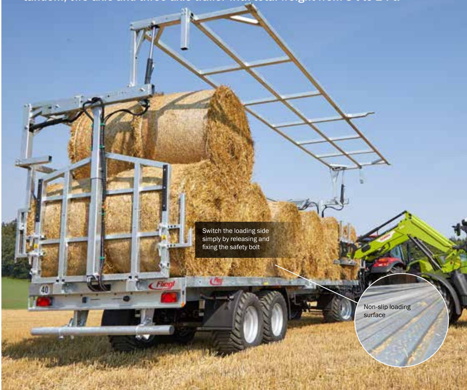
Switch the loading side simply by releasing and fixing the safety bolt
