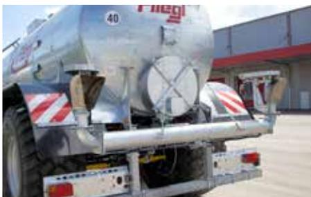
Double pendulum spreader, hydraulic
