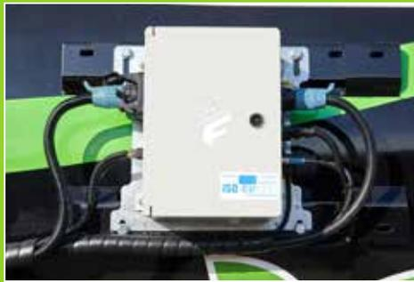
FFC control cabinet with integrated job computer and ISOBUS interface
