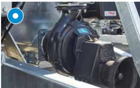
Centrifugal pump for transferring
