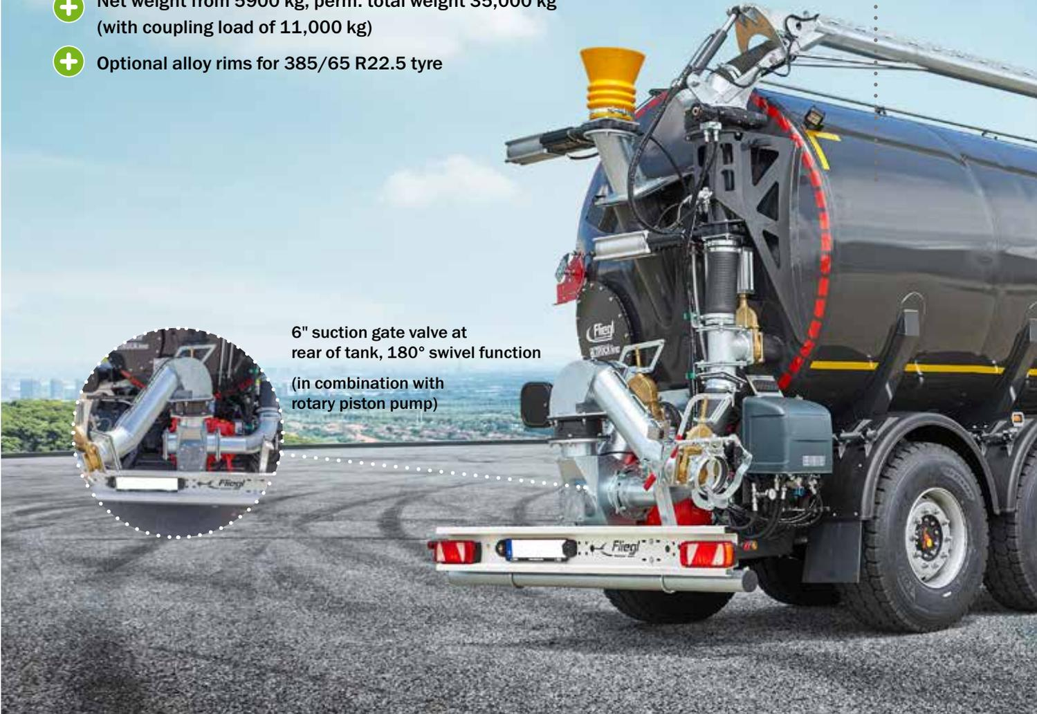
6" suction gate valve at rear of tank, 180° swivel function (in combination with rotary piston pump)
