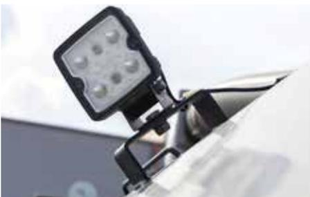
Working light for illuminating the spreader
