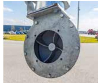
Transfill suction boom – operated via Joystick control. Proportional operation. Approx. 10 m fully extended. Flexible application thanks to robust slewing ring and three joints. Turbo filler at end of boom for outstanding suction performance.
