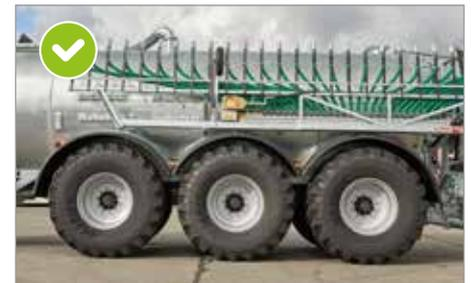
Individual wheel arches in combination with hydr. suspension
