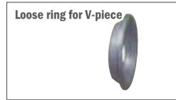
With this system, levers are **welded to the M-piece**. The **V-piece features a ball with a loose clamping ring**. This ring must have a sharp edge where the levers of the M-piece engage. If this edge is rounded, this is known as the »Bazzoli Siegperle« system.
