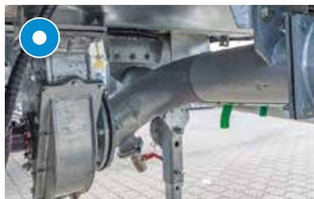
Hydraulic turbo filler, centrally under tank
