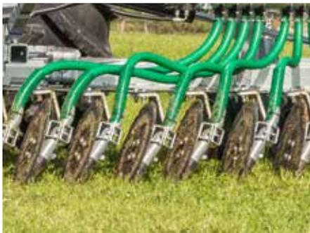
Infinite adjustment of discs
