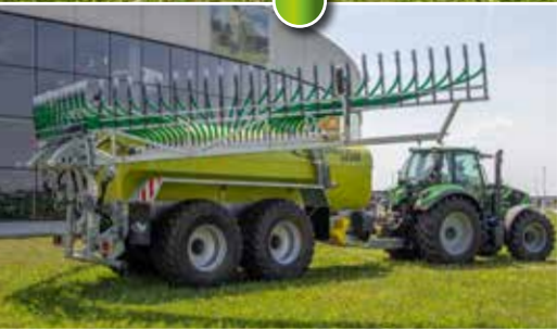
Special folding mechanism prevents any kinking of the outlet hoses
