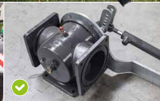
Tapered three-way gate slider with mechanical flow adjustment
