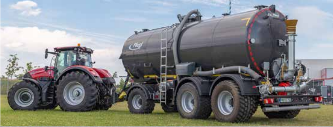
STF 27500 tanker trailer with integrated dolly
