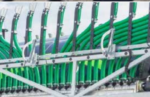
Holder for suction line (shown here in the folded-up state)
