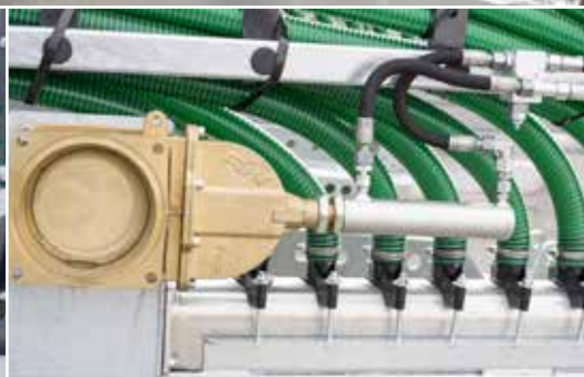
Hydraulic emptying of trap box
