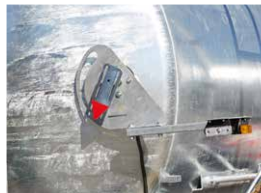
Fill level indicator with float ball
