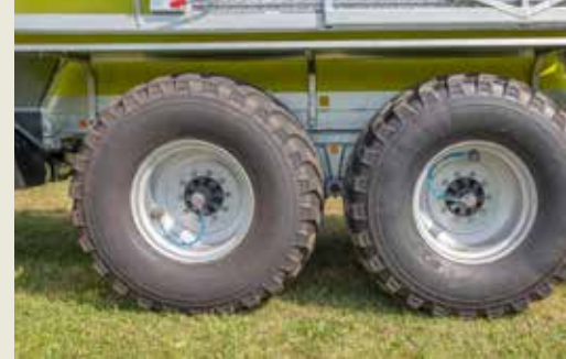
Tyre pressure control system for soil-friendly field applications, with one/two wire system
