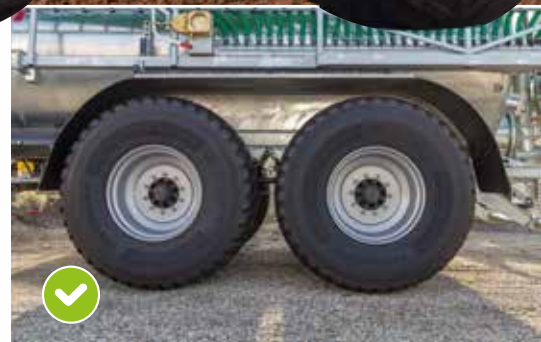
Wheel arch and tyres Tyres 750/60-R30.5“ Optional: Rear tyres 750/60-R30.5“ Front tyres 850/50-R30.5
