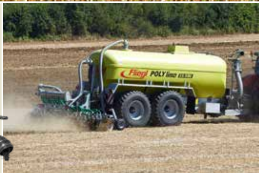
PFW 15,500 with "mole" slurry disc harrow 6 m
