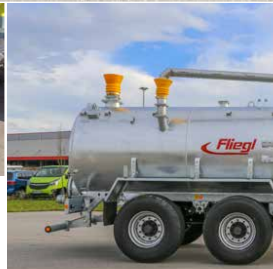
HFW 16,000 Tandem with centrifugal pump and transfer arm, swivels to either side
