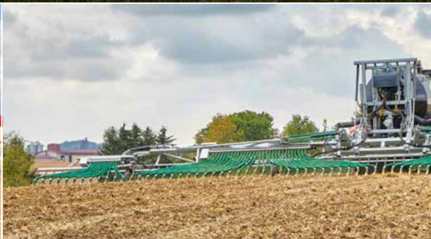
Fliegl SKATE 210 with pendulum frame for better slope compensation (only for SKATE 210/240)
