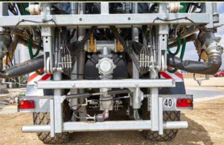
Fliegl SKATE 210 with pendulum frame for better slope compensation (only for SKATE 210/240)
