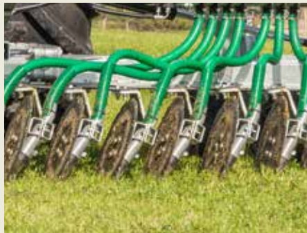
Because of the slanted position of the discs, the soil is opened up so that the slurry can be directly injected
