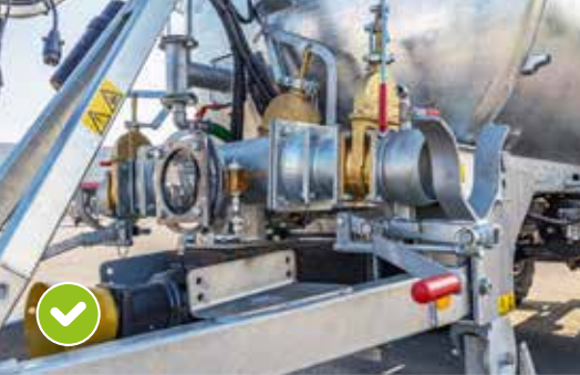
Suction manifold with sight glass
