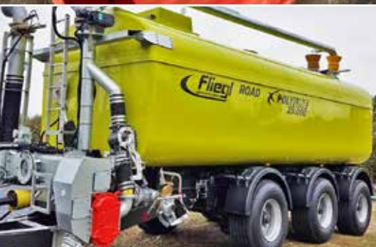
Road X Poly Line with mechanically driven rotary lobe pump for suction
