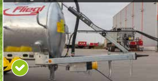
Tank tipping cylinder with drop support leg starting from 5000L
