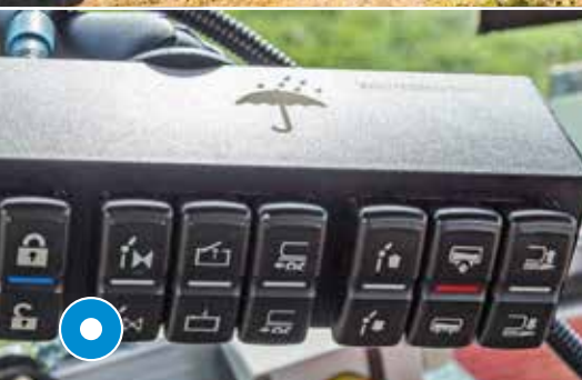
Control panel for tank + distributor Illustration: Red flashing light to protect the pump from running dry
