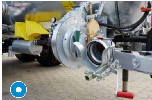
Turbo filler with quick coupler
