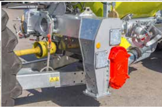
Road X Poly Line with mechanically driven rotary lobe pump for suction
