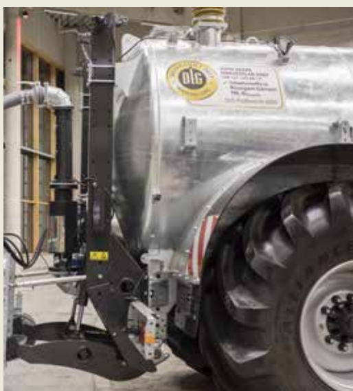
Four-point hydraulics with lifting force 4,500 kg
