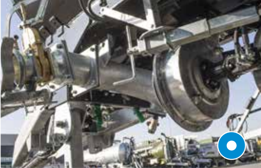
For vacuum tank: Turbo filler at centre under tank
