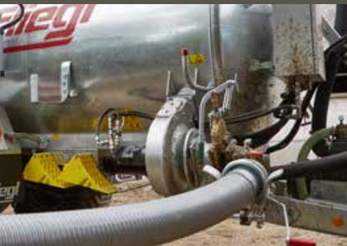
Turbo filler with quick coupler (6" or 8")
