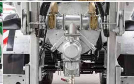
T-piece for an additional outlet (e.g. for a baffle plate spreader) in combination with lateral shut-off.
