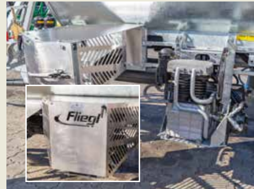
Piston compressor with up to 3.3 m 3 air output
