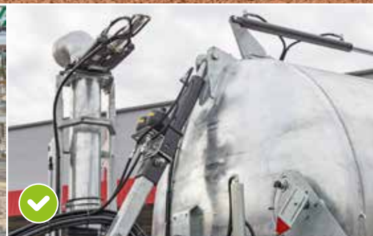
Hydraulic drawbar suspension
