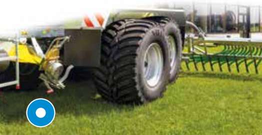
Telescopic axle (only possible with Boogie SB floating assembly)
