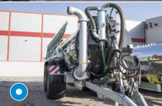
Suction nozzle – to left or right – for easy suction
