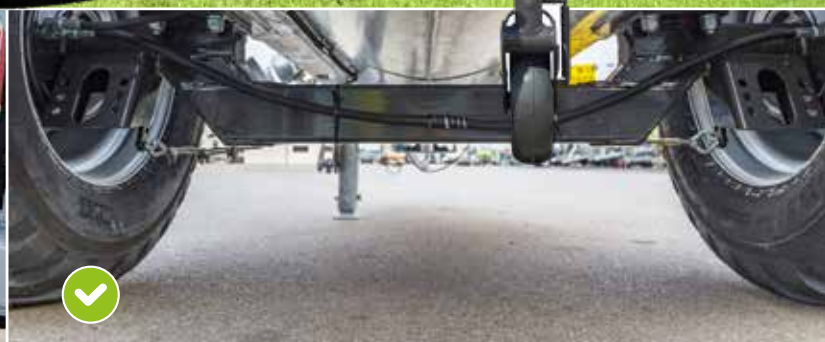
With offset axle starting from 5000 litre: Low centre of gravity ensures optimal handling on slopes
