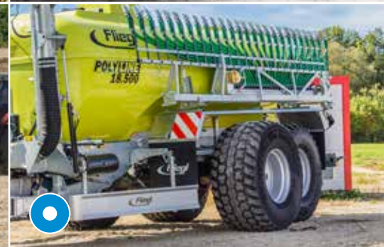
PolyLine available in numerous equipment variants, e.g. with telescopic axle
