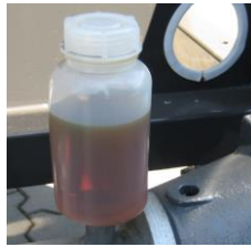
Fig. 16: Oil container for lubricating the flushing pump
